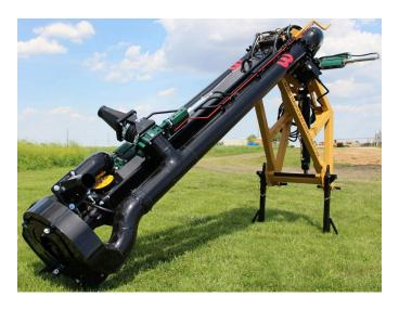
24. Lastly, Bazooka advertises that the Riptide Manure Pumps include "dual, independent nozzles" that direct liquid from the pump into the manure lagoon for agitating the lagoon. The nozzles also contain a valve for controlling a liquid manure flow rate through the nozzle. (https://www.bazookafarmstar.com/wp-content/uploads/2021/06/IMG\_1652-1024x683.jpg).
